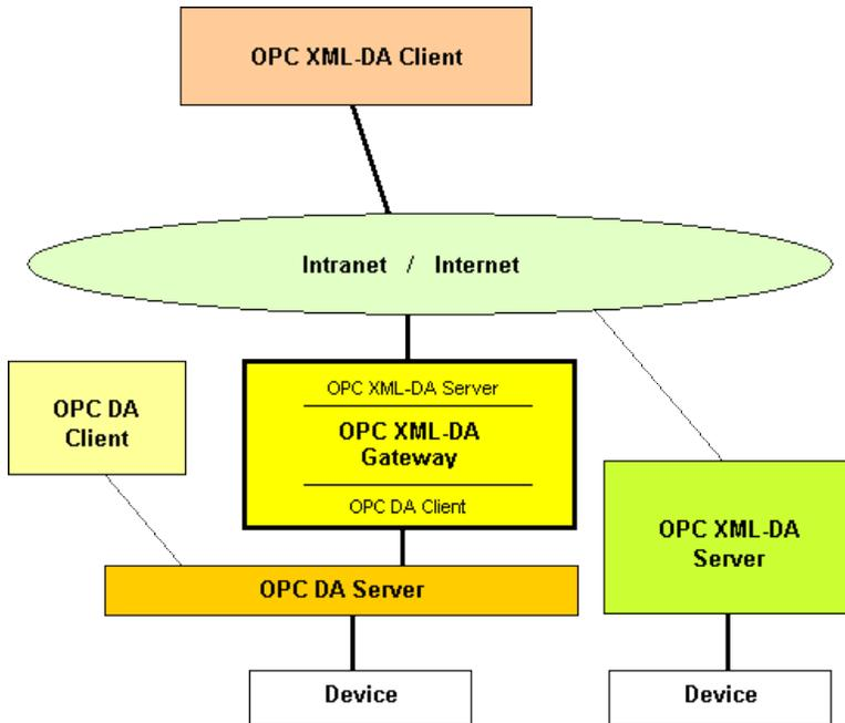
The XDAGW-SS Gateway software package consists of the following components:
